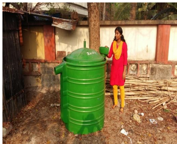
Installation of Kitchen waste processing unit nearby Canteen of main campus of Calicut, CMFRI for biogas generation for cooking on 31.10.16
